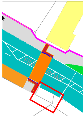
Figure 2-9: Absence of Warning Tactiles (Drawing 11199-08-1010-B)
